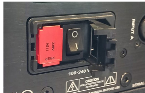
Step 4: Insert the fuse holder ensuring it is fully engaged.
