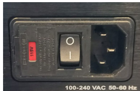
Step 5: Push the fuse holder cover in so that it is completely sealed.
