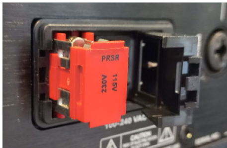
Step 3: Remove the fuse holder and rotate so that the voltage rating you require is oriented to the left.
