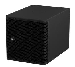
This single 15" reflex-loaded low frequency enclosure delivers a frequency response of 38 Hz - 160 kHz  $\pm$ 3 dB and efficiency of 97 dB. Features include a tough 15" high excursion transducer with a 4" voice coil and a strong enclosure made entirely from 18 mm multi-laminate birch plywood.
