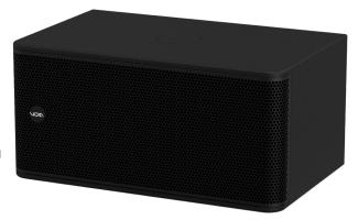
As the Venu 112 V2's big brother, Venu 212 V2 is a double 12" compact low frequency enclosure offering a frequency response of 34Hz – 160Hz ±3 dB and efficiency of 99dB. Features include two tough 12" high excursion transducers with 4" voice coils and a sturdy enclosure made entirely from 15 mm multi-laminate birch plywood.
